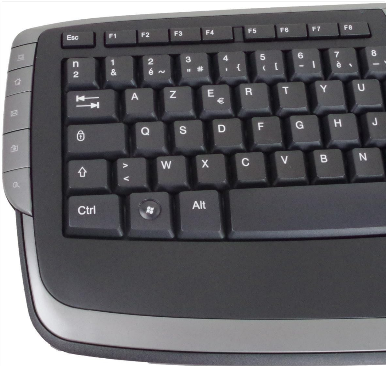
Image 2: Close-up view of the left side of the keyboard, highlighting the Azerty key layout (e.g., 'A' key, 'Z' key) and the dedicated shortcut buttons on the left bezel.
