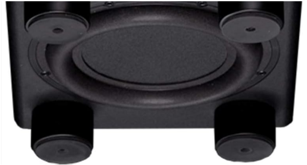
Figure 3.3: Bottom view of the TS107, revealing the 6.5-inch passive radiator. This design element contributes to the subwoofer's extended low-frequency response without the typical port noise associated with ported designs.
