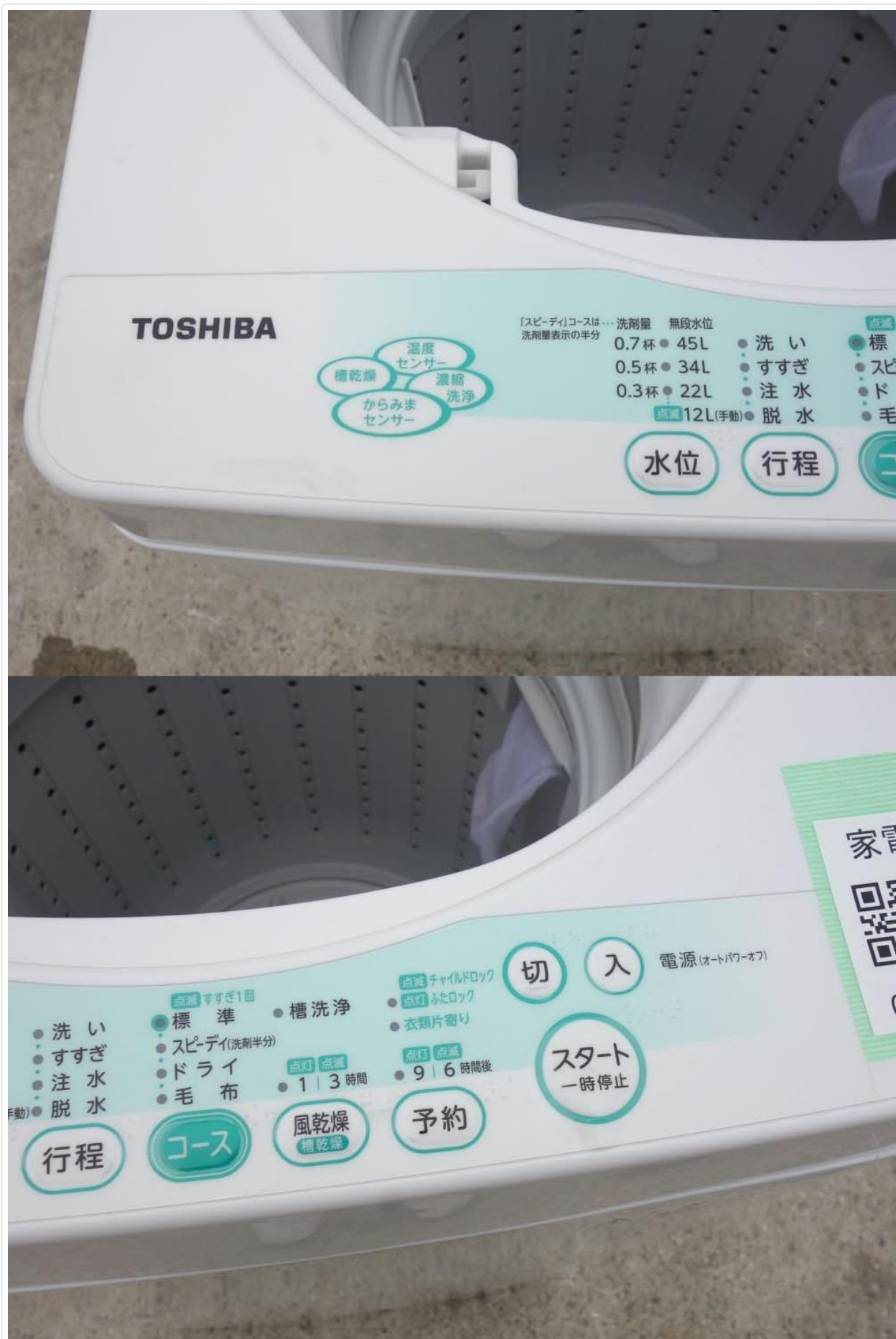
Figure 4.1: Close-up of the washing machine's control panel. Key functions include power (On/Off), Start/Pause, Water Level, Process (Cycle), Course selection, and Delay Start. Indicators for Warm Air Dry Sensor and Tangle Sensor are also visible.
