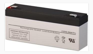
Image: SigmasTek FP1223 12 Volt 2.9 AmpH Sealed Lead Acid (SLA) battery. The battery is rectangular, white with a black top, and features F1 terminals on the top. Text on the battery casing indicates it is a 'Rechargeable Sealed Lead-Acid Battery (12V2.9AH/T1)' and provides 'CHARGING INSTRUCTION' details: 'Floating use: 13.5-13.8V', 'Cycle use: 14.4-15.0V', 'Initial current: max 0.87A'. Recycling symbols and a UL certification mark are also visible.
