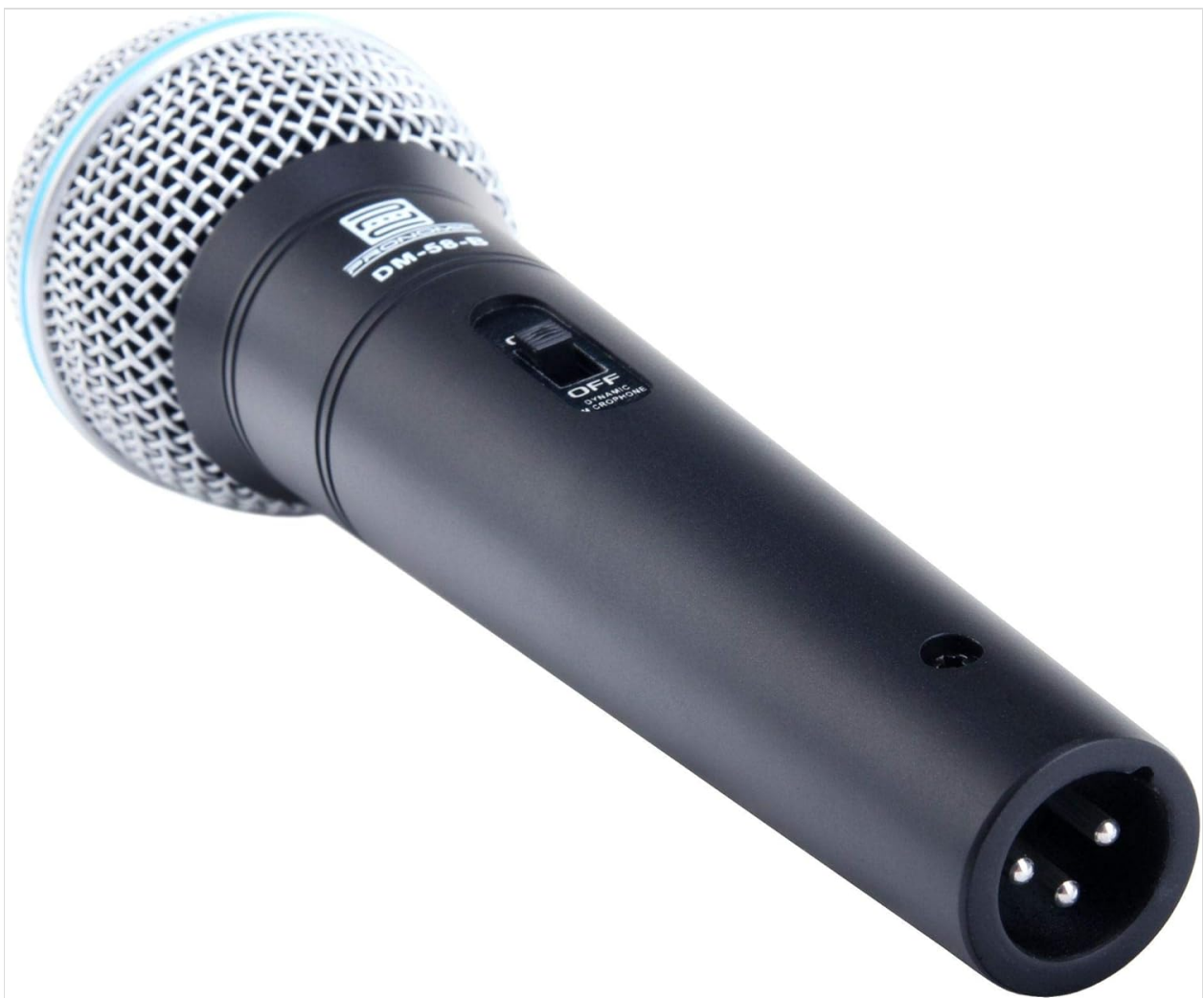
Figure 2.3: Bottom view of the microphone, showing the 3-pin XLR output connector.
