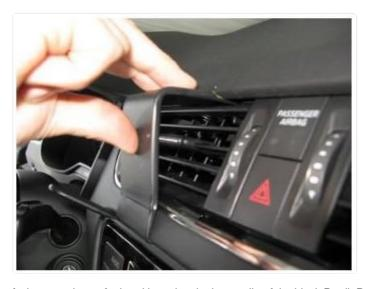
**Image Description:** A close-up photo of a hand inserting the bottom lip of the black Brodit ProClip into the seam between the dashboard and the air vent assembly, to the right of the steering wheel.
