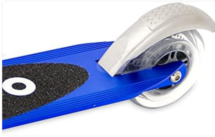
Figure 5.1: Detail of the rear wheel and fender brake.
