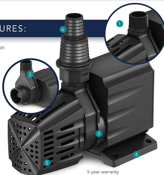
Figure 1: Detailed diagram highlighting the key features of the Atlantic MD-Series pump, including its oversized male threaded inlet/outlet, rotating volute, quarter-twist volute access, large stable base, removable pre-filter, and tapered outlet fittings. A 5-year warranty is also noted.
