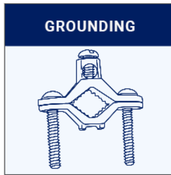
Image 5.3: Illustration depicting a grounding connection, similar to how the lay-in lug secures the grounding wire.
