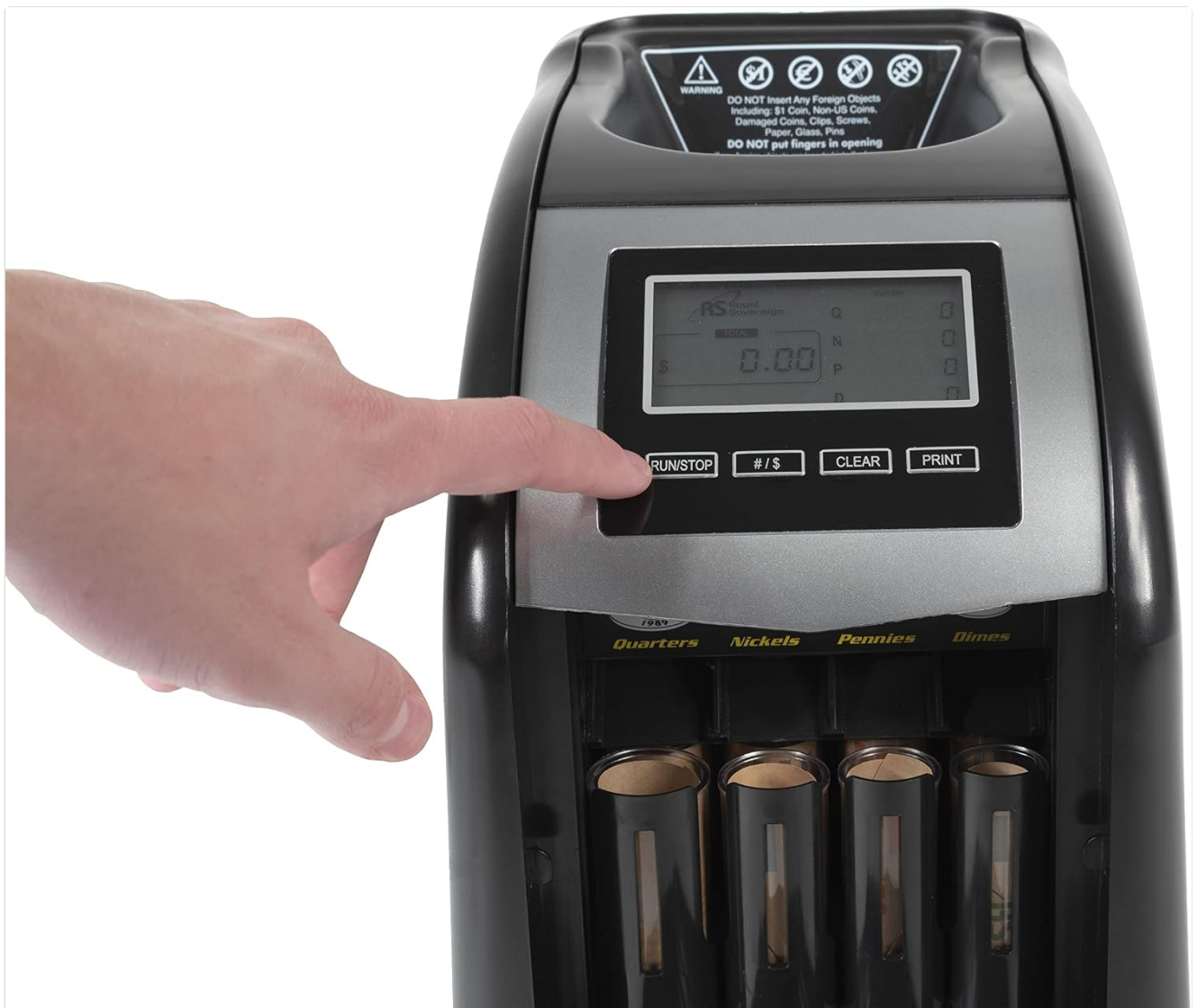
Figure 6: Initiating the sorting process.
