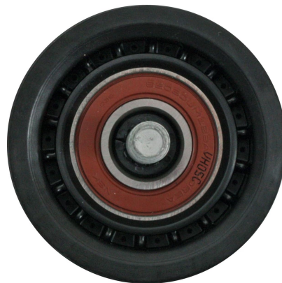
Rear view of the pulley, showing the bearing and its housing.
