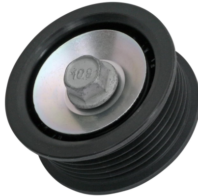
Front view of the Continental 50016 Accu-Drive Pulley, showing the ribbed surface and mounting bolt.
