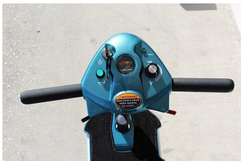
Figure 3: Detailed view of the scooter's control panel, including the key slot, battery charge indicator, and speed adjustment dial.
