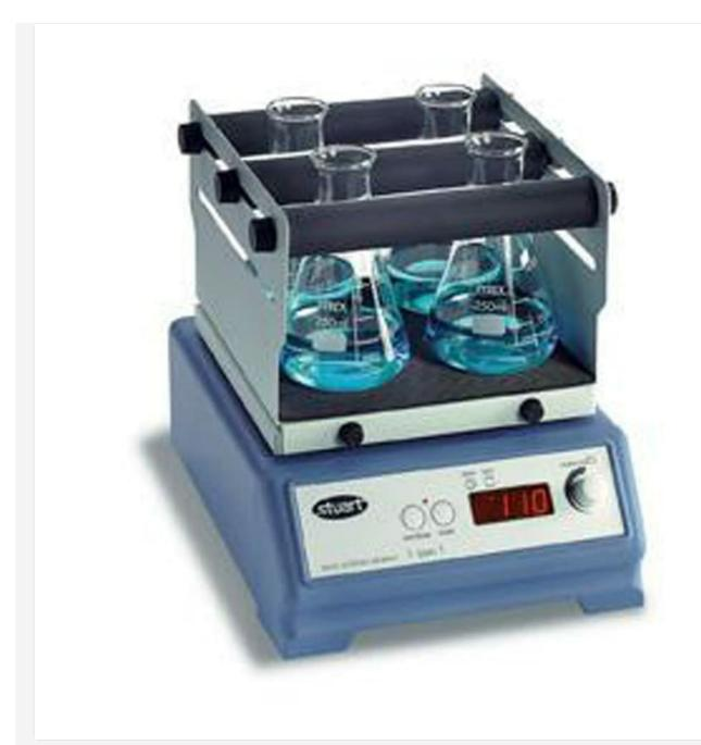
Figure 4: Stuart SSM1 Mini Orbital Shaker with four 250ml Erlenmeyer flasks secured in the accessory cradle system, illustrating a common setup for medium-sized flasks.
