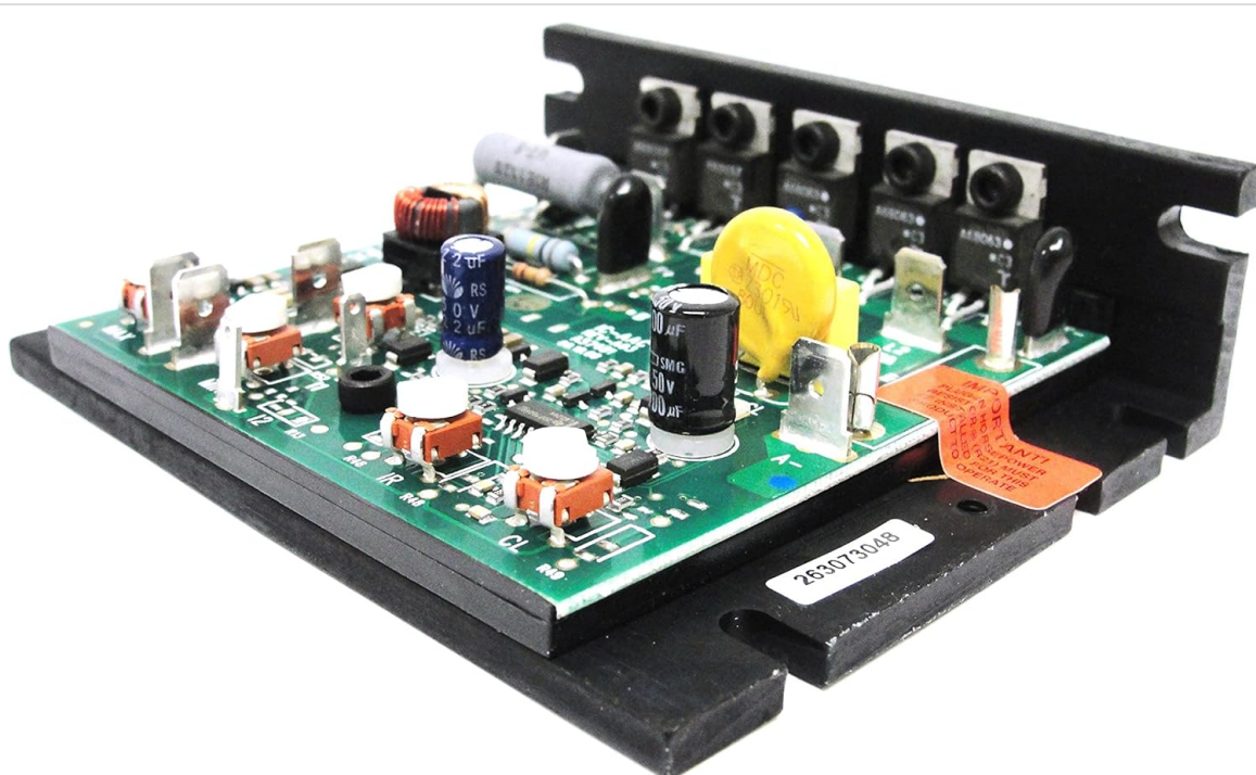
Figure 3.1: Angled view of the KBIC-240D control board, highlighting its compact design and electronic components.
