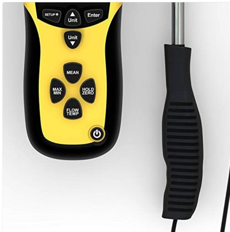
Image 2: Detailed view of the TA300 control buttons and LCD display.
