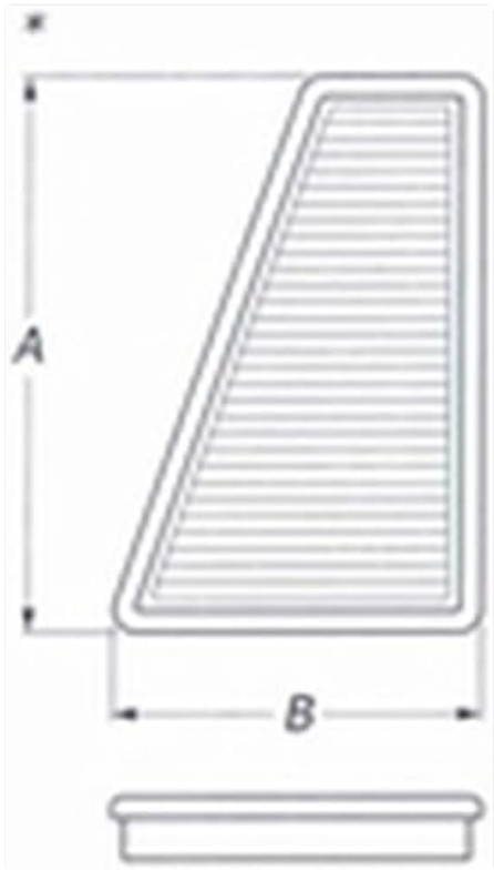
Figure 3: Schematic diagram illustrating typical dimensions (A and B) for a panel air filter, similar to the FB156/01 model.
