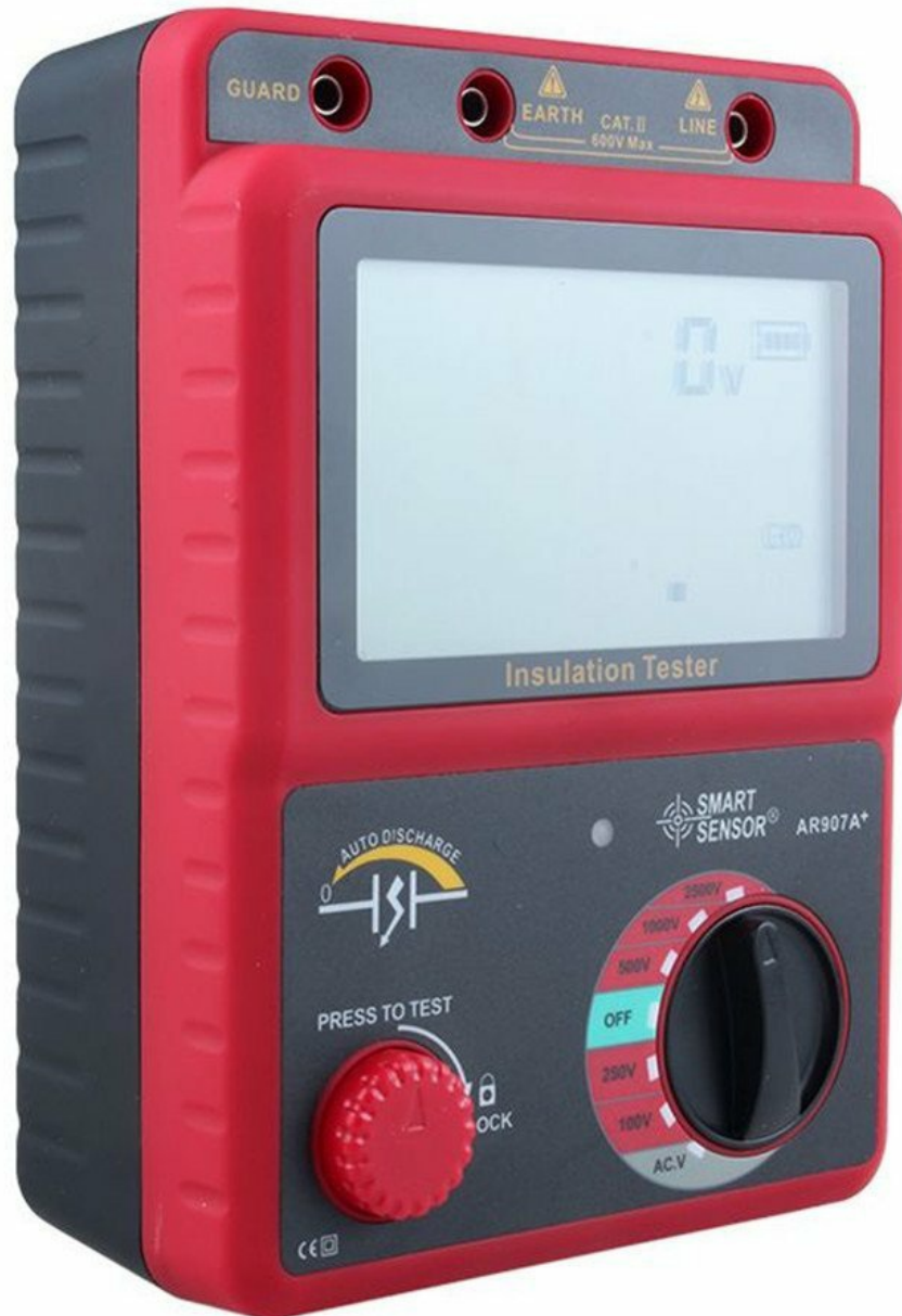
Figure 1: Front view of the SMART SENSOR AR907A+ Insulation Tester, showing the display, control knob, and test button.
