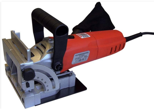
Figure 4: Detail of the turret stop for depth adjustment, enabling quick selection for lamella sizes 0, 10, and 20.
