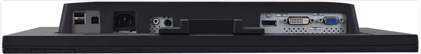
Figure 3: Connectivity ports on the rear of the monitor, including DisplayPort, DVI, VGA, Audio, USB, and Power.
