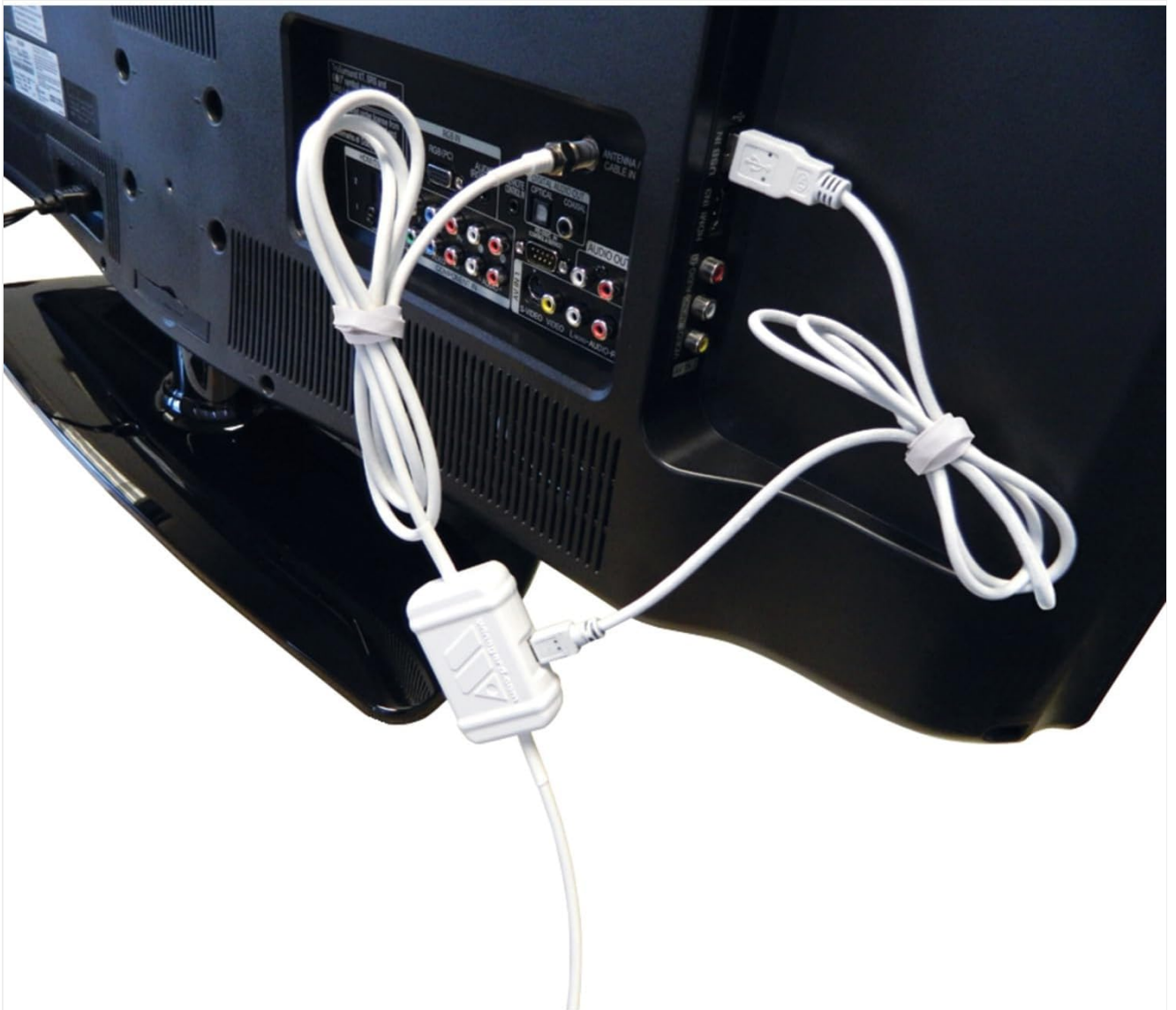
Image: Close-up view of the antenna's coaxial cable and amplifier connected to the back of a television via the 'Antenna In' port and a USB port for power.
