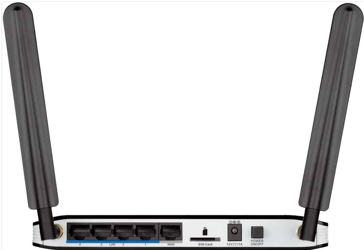
Image: Rear view of the D-Link DWR-921_E router, showing the power port, SIM card slot, WAN port, LAN ports, and antennas.
