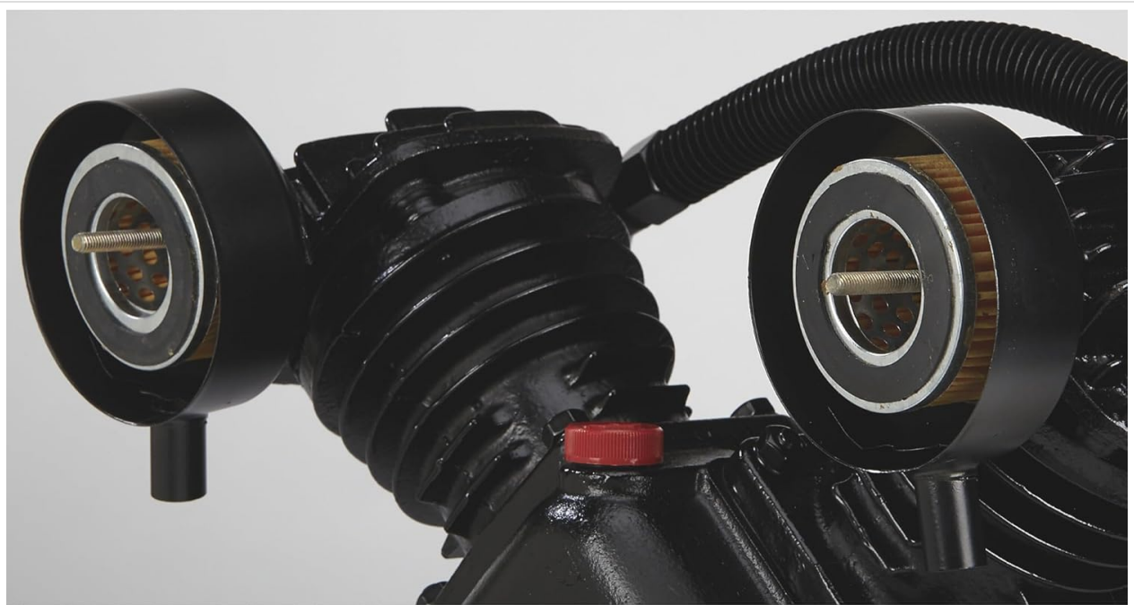
Figure 3: Close-up of the air intake filters, which should be kept clean.
