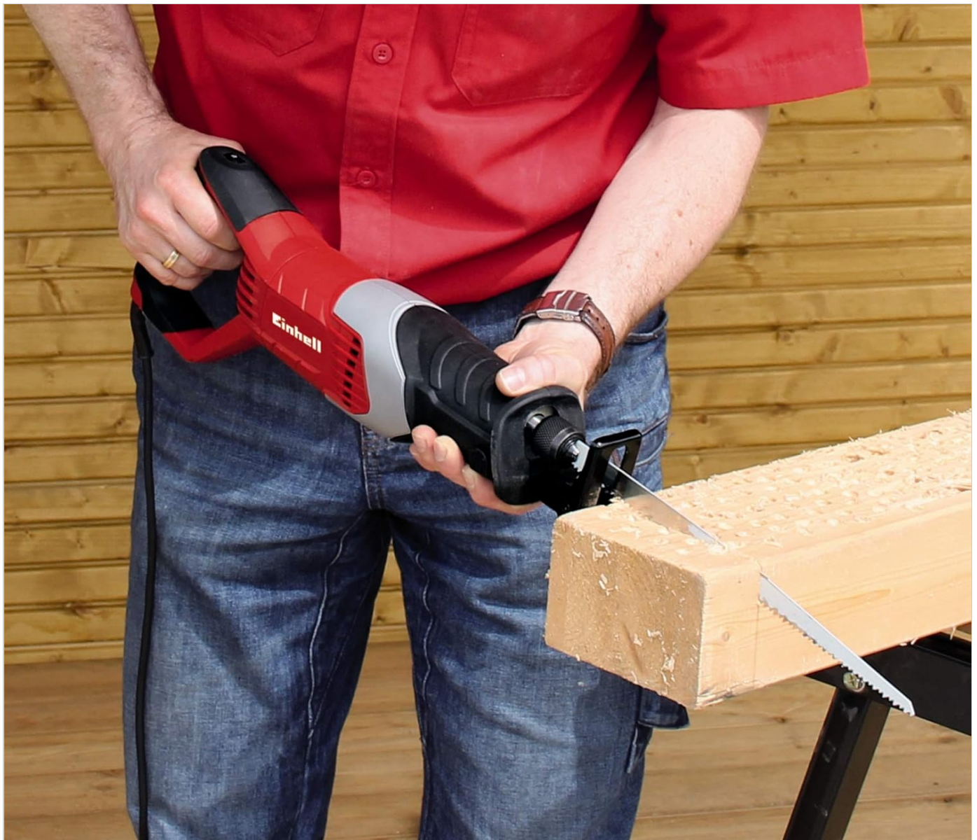
Figure 6: A user demonstrating the operation of the reciprocating saw, cutting a wooden beam. Always ensure proper grip and workpiece stability.
