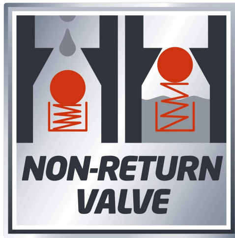
Figure 9: Diagram illustrating the function of the non-return valve, preventing backflow.
