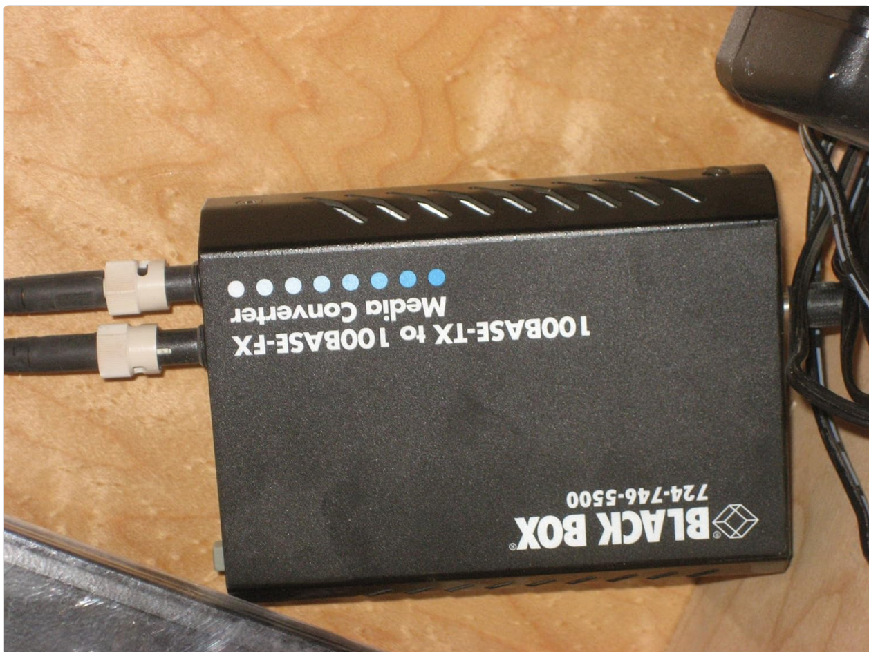
Figure 1: Black Box 724-746-5500 Media Converter. The image shows the black rectangular device with two fiber optic cables connected to the left side. The top surface displays the text "100BASE-TX to 100BASE-FX Media Converter" and the Black Box logo with part number "724-746-5500". Several small indicator lights are visible on the front panel.
