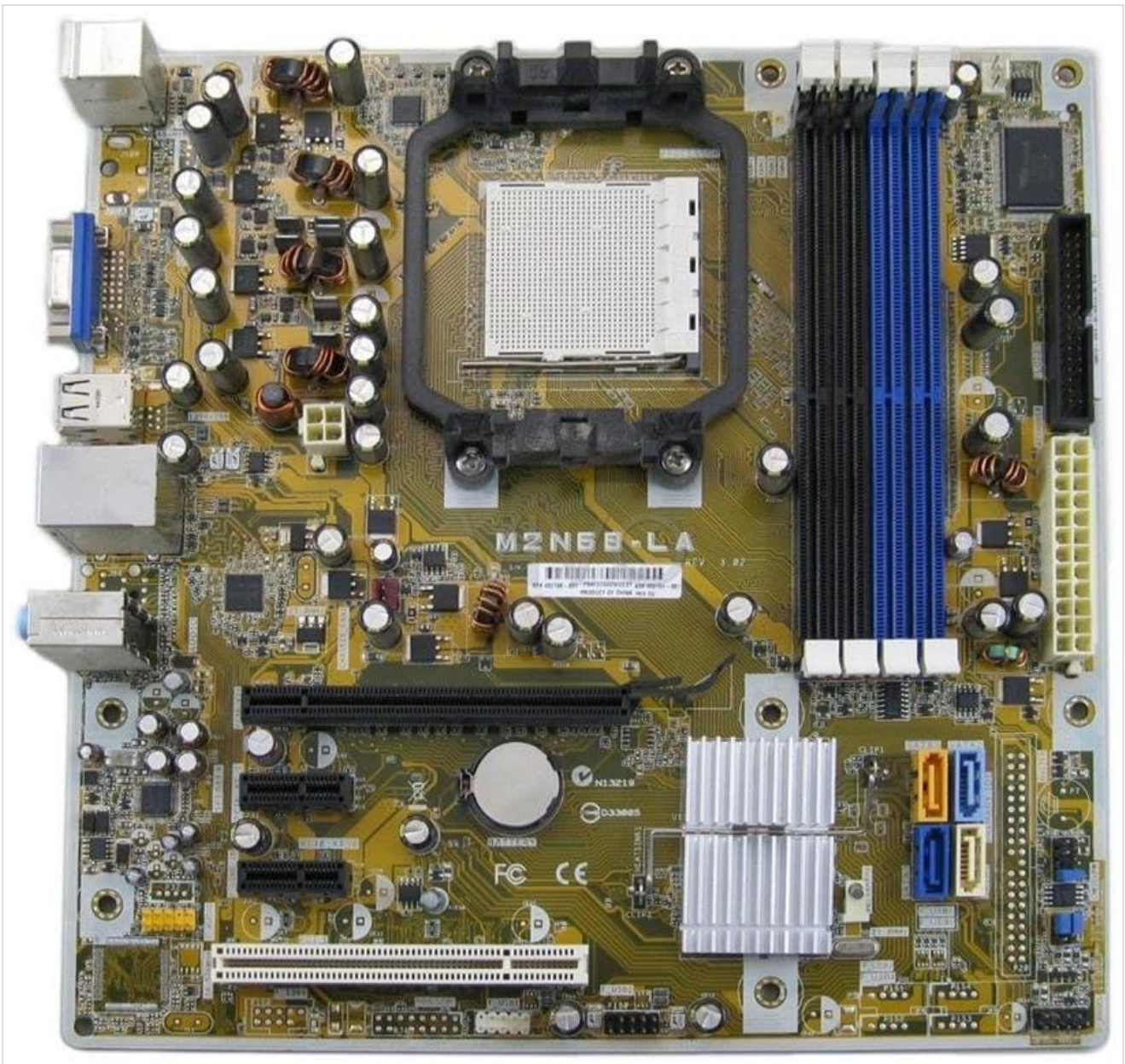
Figure 1: Top-down view of the HP M2N68-LA Motherboard. Key components visible include the CPU socket (center), four DDR2/DDR3 RAM slots (blue and black, right), PCI Express and PCI slots (bottom), SATA ports (orange/blue, bottom right), and various power connectors and headers.
