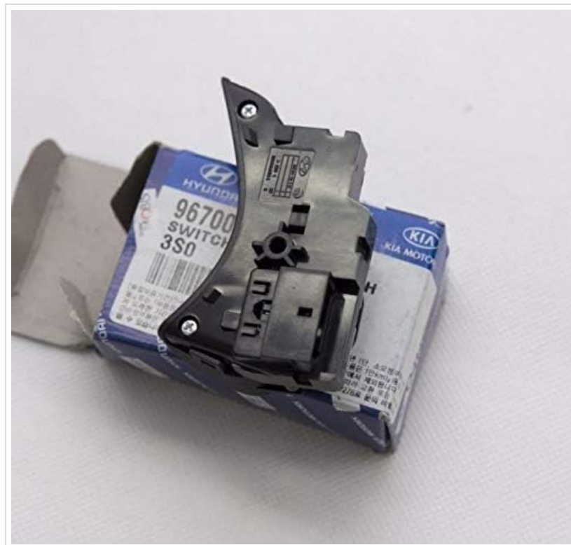
Figure 1.2: A rear view of the Hyundai 96700-3S900-RY Steering Switch Assembly. This perspective shows the mounting points and electrical connectors, crucial for proper installation and ensuring a direct fit within the vehicle's steering column.
