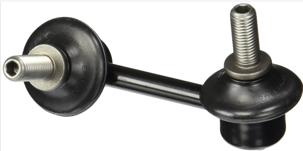
Image 1: The Genuine Honda 52320-SNA-A01 Right Rear Stabilizer Link. This image displays the complete stabilizer link, featuring the central bar and the two ball joint ends with threaded studs for attachment to the vehicle's suspension system. The black rubber boots protect the ball joints, and the metal studs are visible, one with a hexagonal recess for an Allen key to prevent spinning during tightening.
