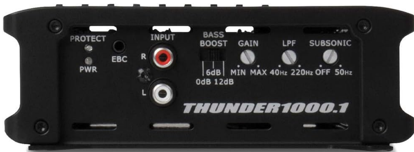
Figure 3: Input and Control Panel.
