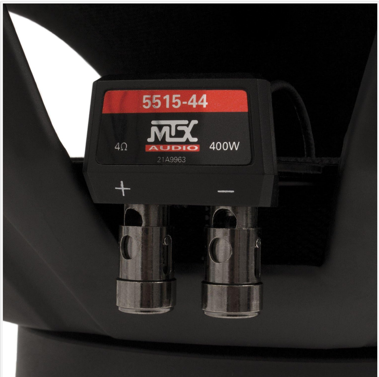
Figure 3: Detailed view of the dual 4 Ohm wiring terminals on the subwoofer, showing positive (+) and negative (-) connections.
