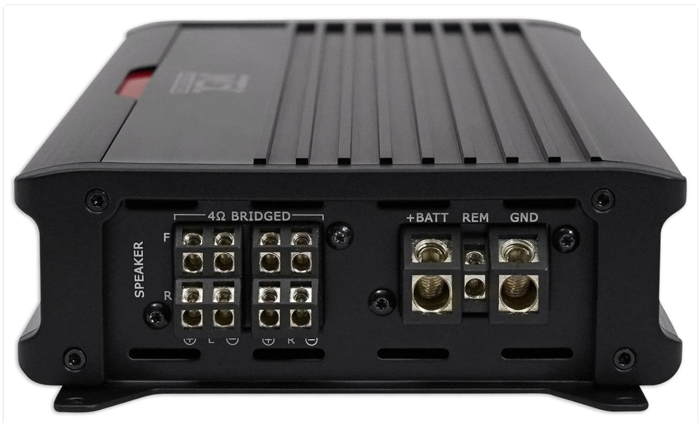
Figure 4.3: Rear panel showing GND (Ground), +BATT (Power), REM (Remote Turn-On), FUSE, and SPEAKER terminals. Note the 4Ω BRIDGED markings for speaker connections.
