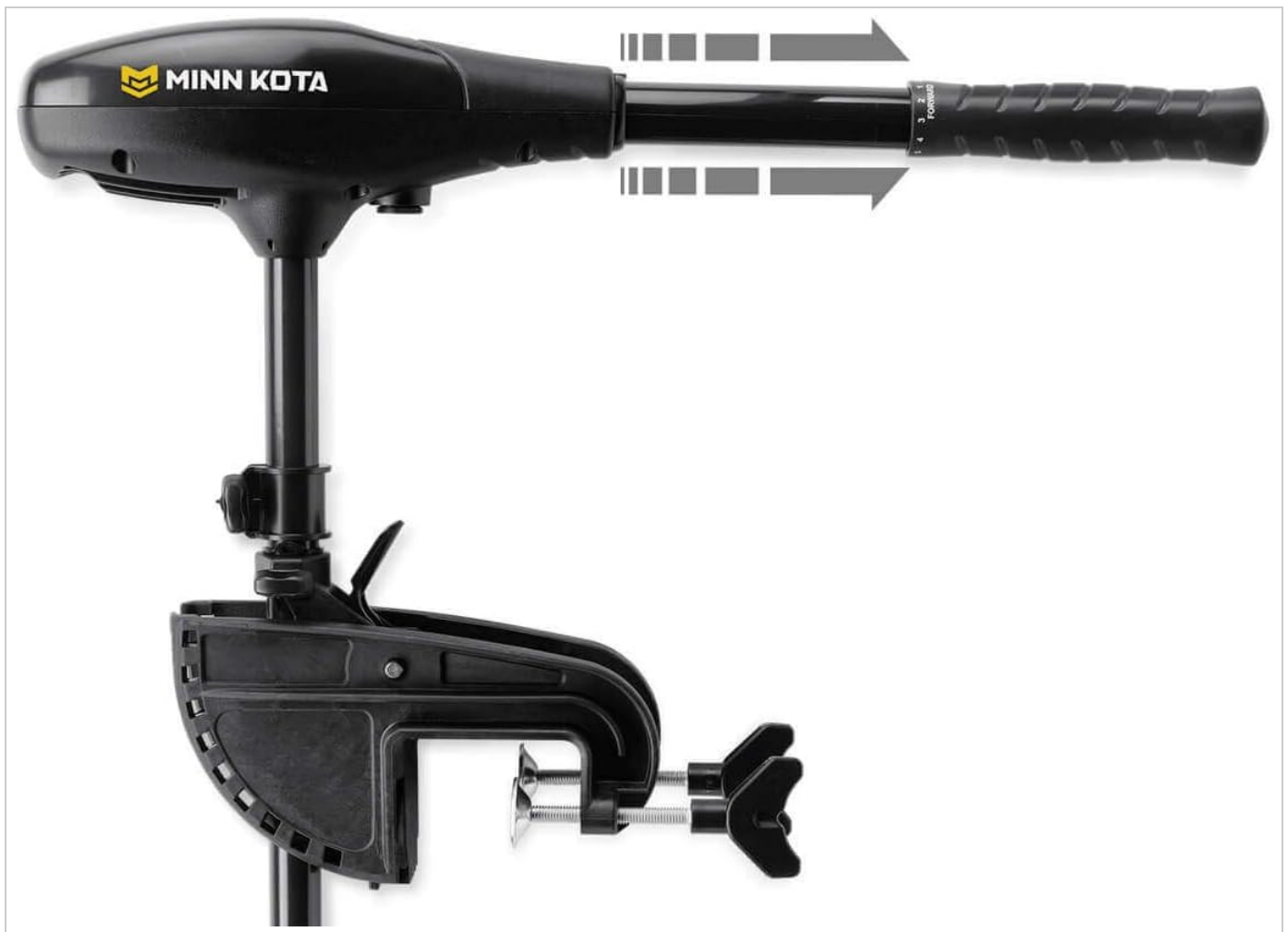
Figure 5: The telescoping tiller handle, which extends for comfortable and intuitive operation.
