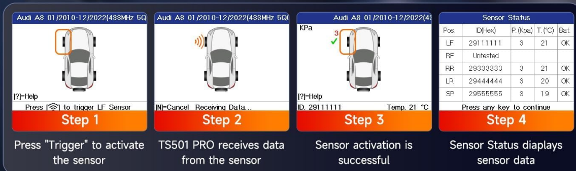
Figure 6.1: Steps for activating a TPMS sensor and viewing its data on the TS501 PRO display.
