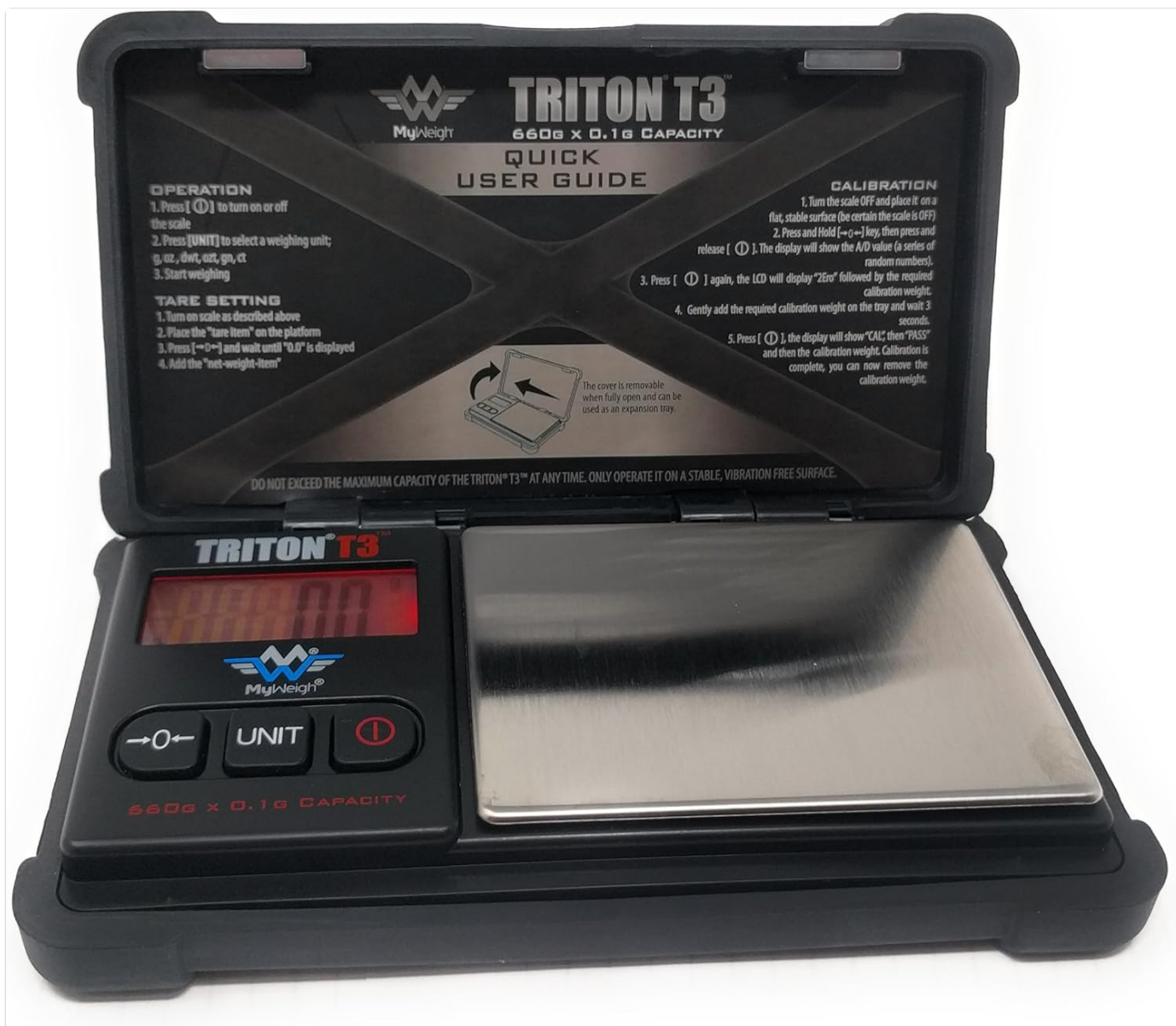
Figure 1: My Weigh Triton T3 Digital Scale in open position, revealing the stainless steel weighing platform and the digital display. The inside of the protective lid features a quick user guide.
