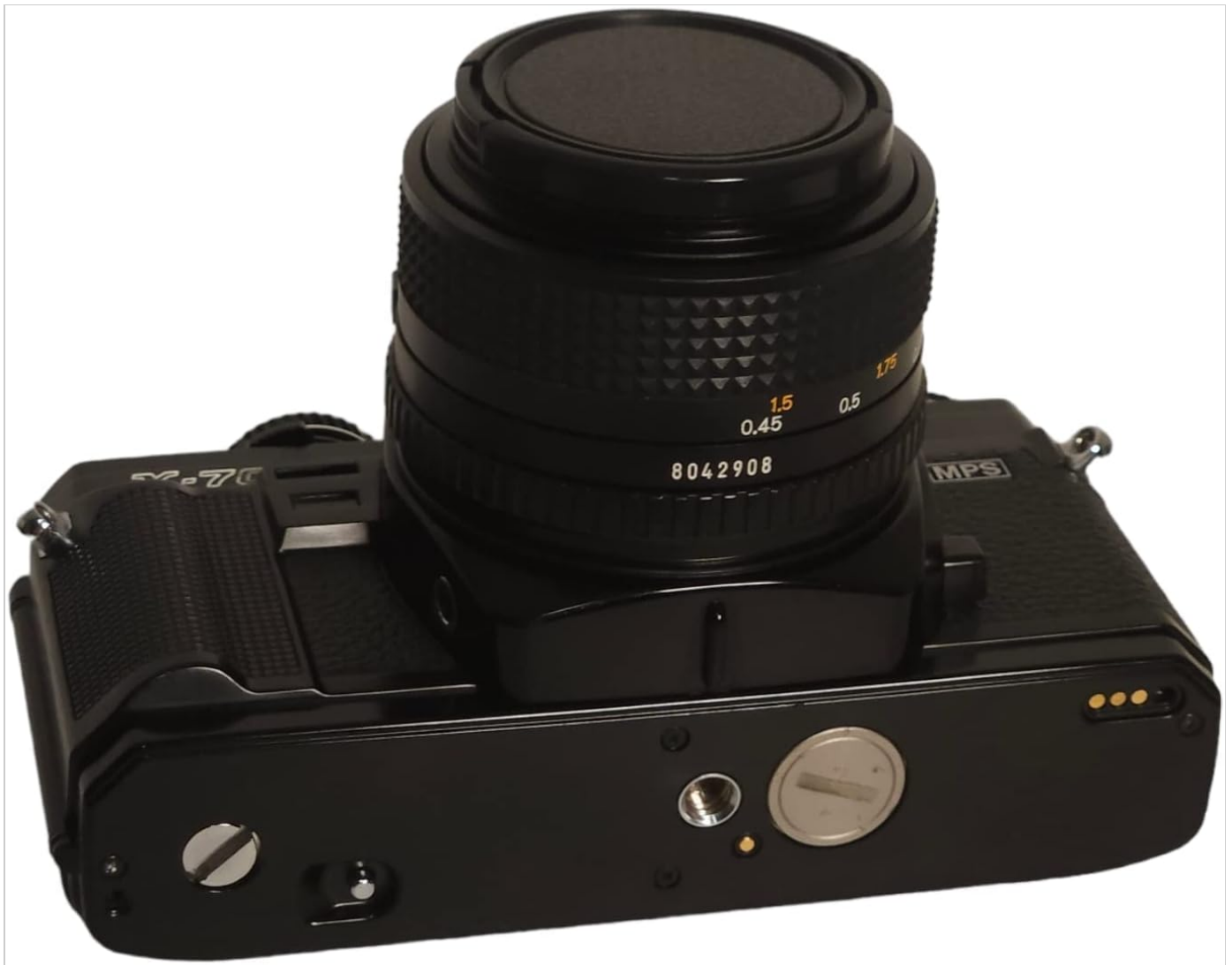
Figure 3: Underside of the Minolta X-700, highlighting the battery compartment and tripod socket.
