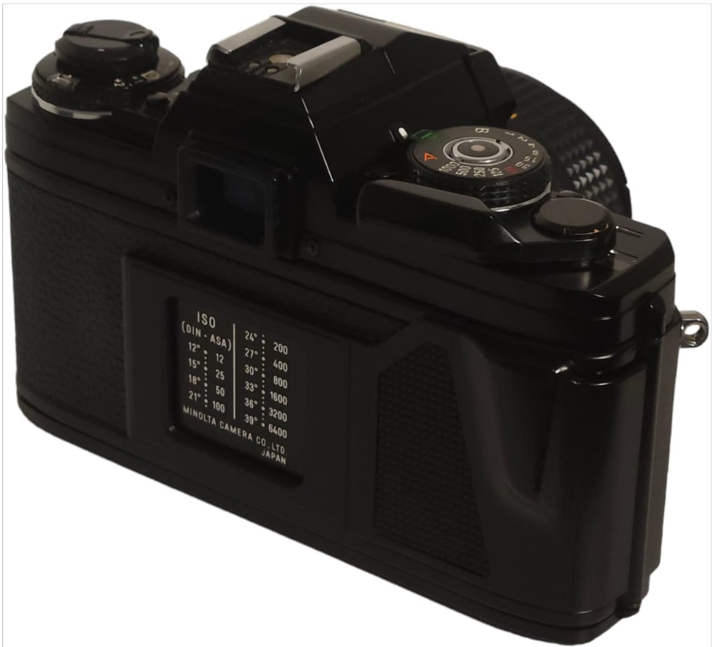
Figure 4: Rear view of the Minolta X-700, displaying the film door and the ISO/ASA setting guide.
