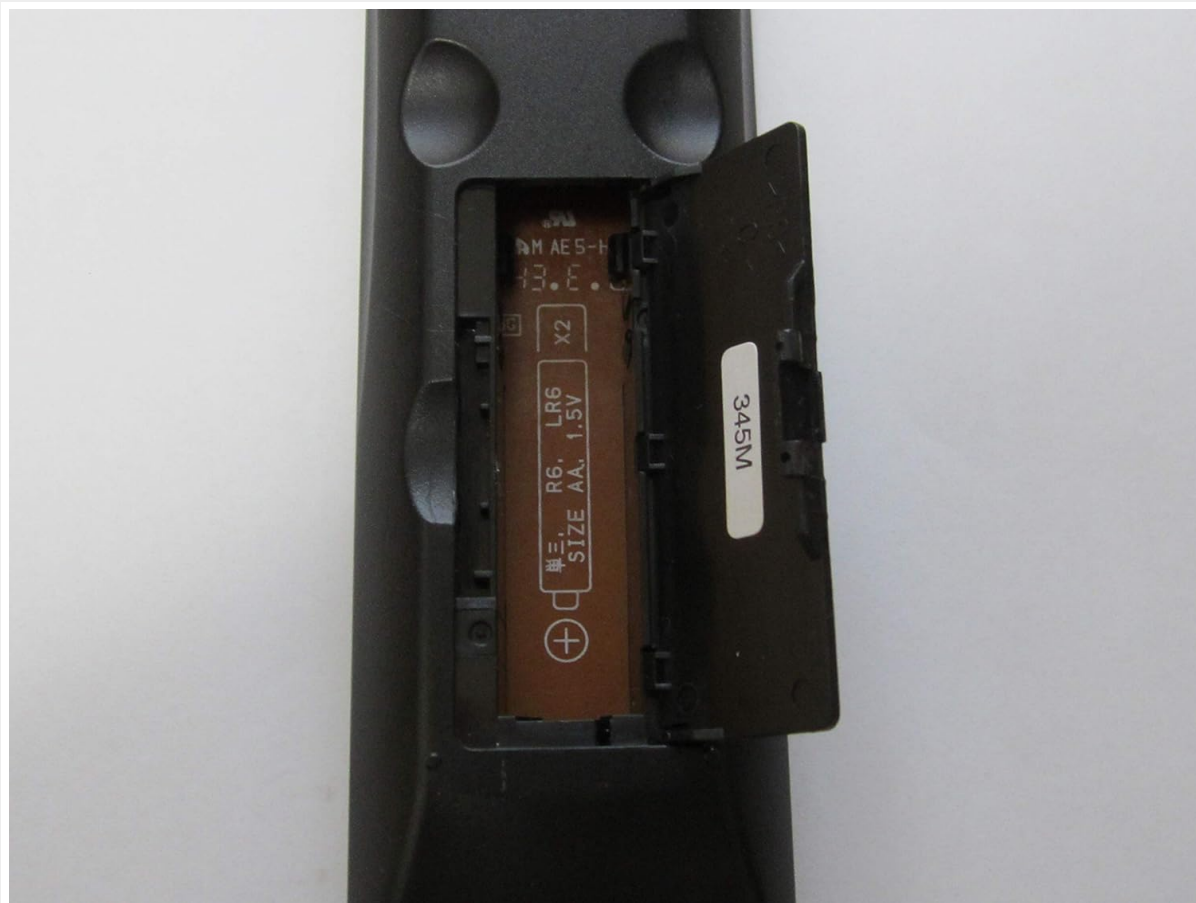
Figure 3: Remote control with the battery compartment open, revealing the slots for two AA batteries and polarity markings.
