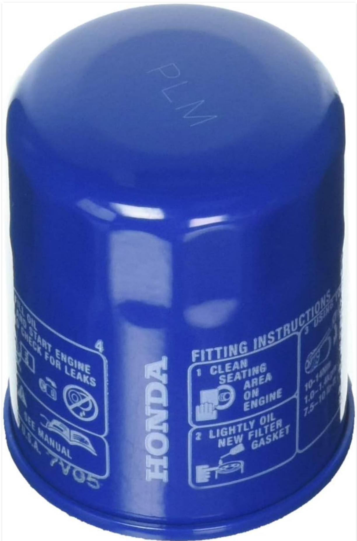
Image: Genuine Honda Marine Outboard Oil Filter. The filter's side displays fitting instructions: 1. Clean seating area on engine. 2. Lightly oil new filter gasket. 3. Tighten using specified torque (10-14 ft-lbs / 7.5-10 Nm). 4. Fill oil, start engine, and check for leaks. The Honda logo is also visible.
