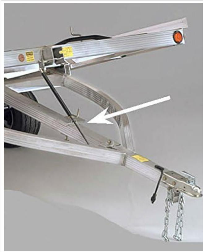
Figure 2: Example of the gas shock installed on a Triton snowmobile trailer. The white arrow indicates the position of the installed gas shock, connecting the trailer frame to the tilting deck.
