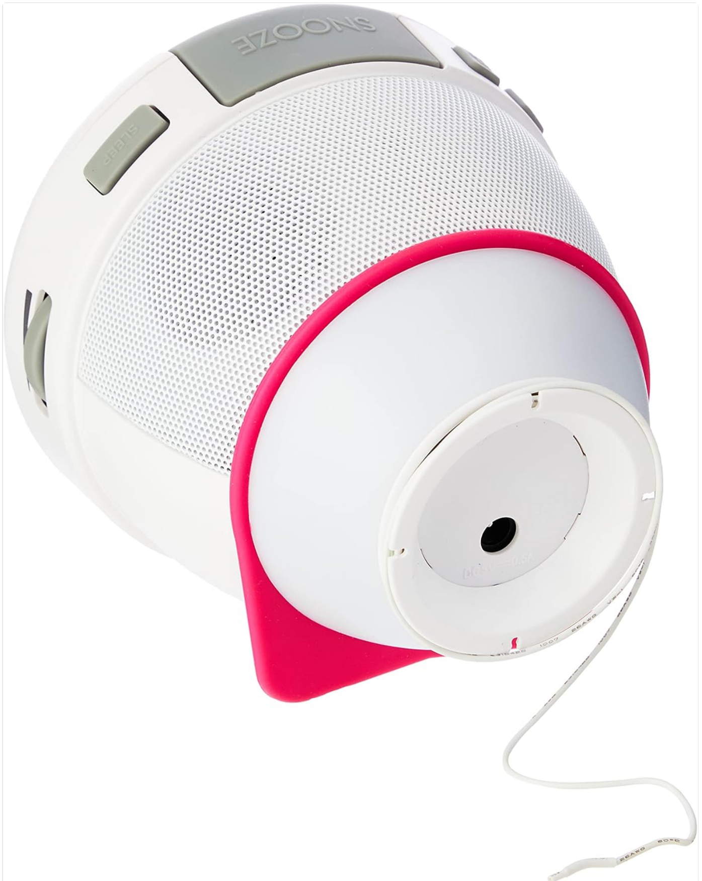
Figure 3: Wake-up Light and Base. This image illustrates the bottom of the Sonoclock 220, revealing the circular base which houses the wake-up light. The power cable is also visible, extending from this section.
