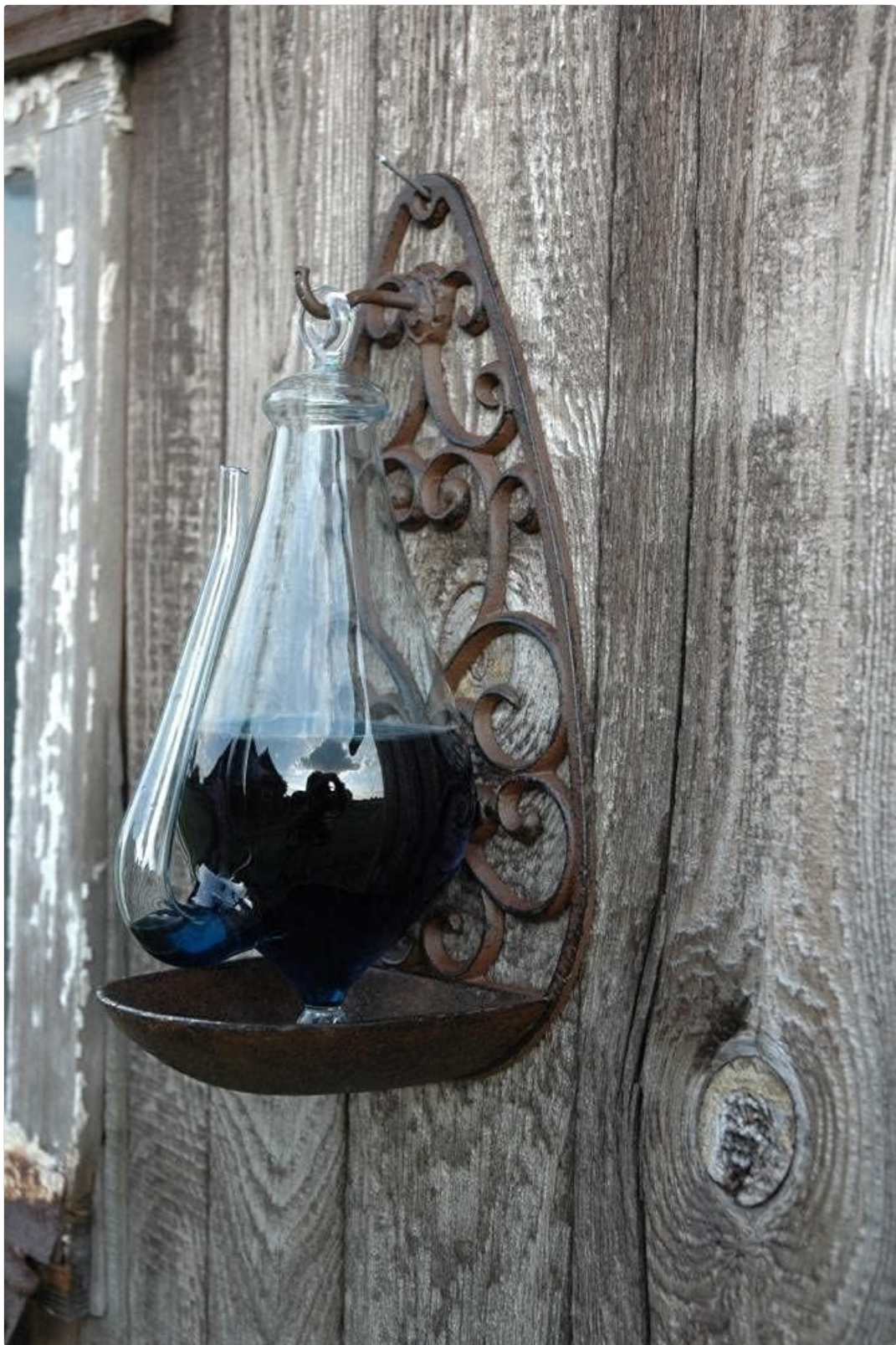
Image: A close-up of the barometer's glass spout, illustrating how the liquid level indicates atmospheric pressure changes.
