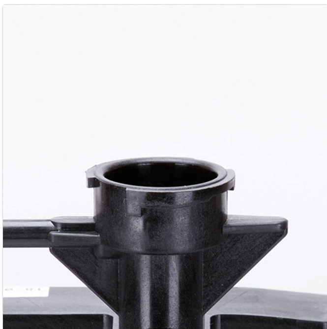
Figure 4: Detail of the radiator fill neck, where the radiator cap is installed.
