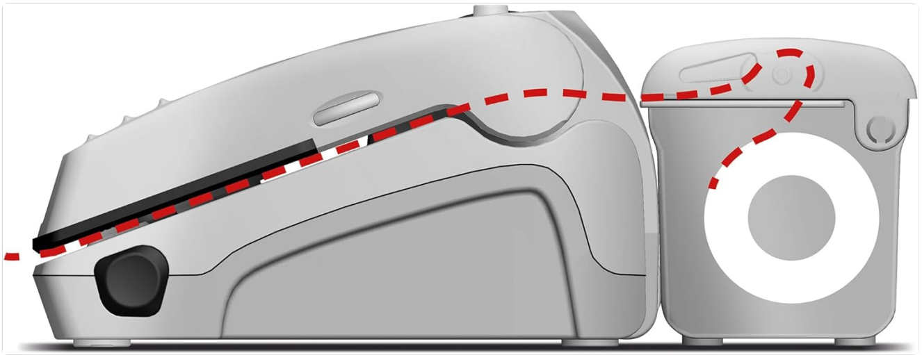
Figure 5: Side view of the unit, showing the connection point for the external vacuum hose used with containers.
