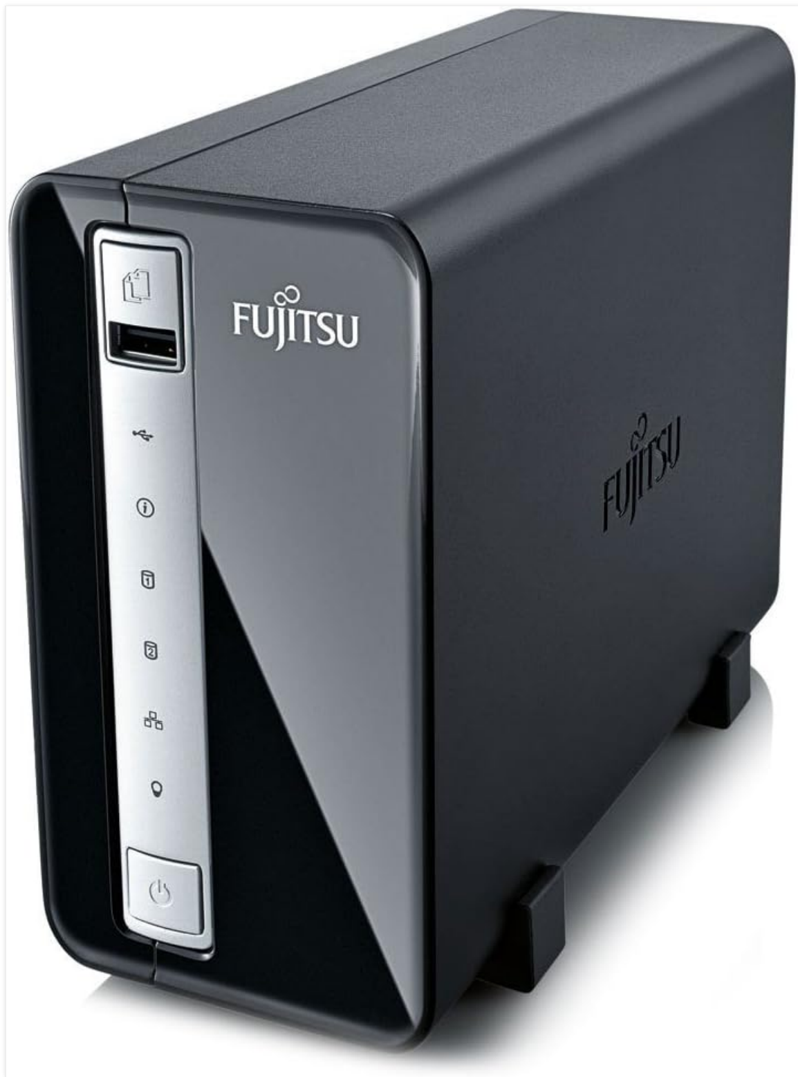
Figure 1: Front view of the FUJITSU CELVIN Q700 NAS server. The device is a compact, dark grey unit with a glossy black front panel. On the left side of the front panel, there's a silver-colored vertical strip containing the Fujitsu logo, a USB port, and several indicator icons for status, network, and drive activity. A power button is located at the bottom of this strip. The overall design is sleek and functional, suitable for a professional or home environment.
