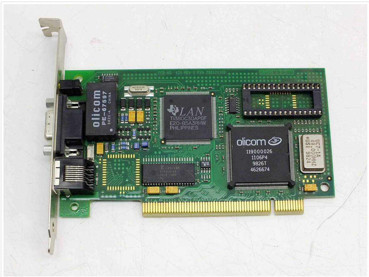
Figure 2.2: Top-down view of the Olicom OC-3137 Token Ring 16/4 PCI Adapter. This image provides a clear view of the PCB layout, including the LAN and Olicom branded chips, and the various electronic components.
