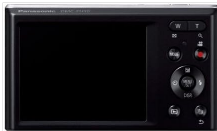
Image 4.2: The rear panel includes the 2.7-inch LCD screen, zoom lever (W/T), Mode button, Video Record button, Menu/Set button, Display button, Playback button, and Delete button.
