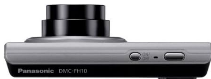
Image 4.3: The top of the camera features the ON/OFF power button and the Shutter button.
