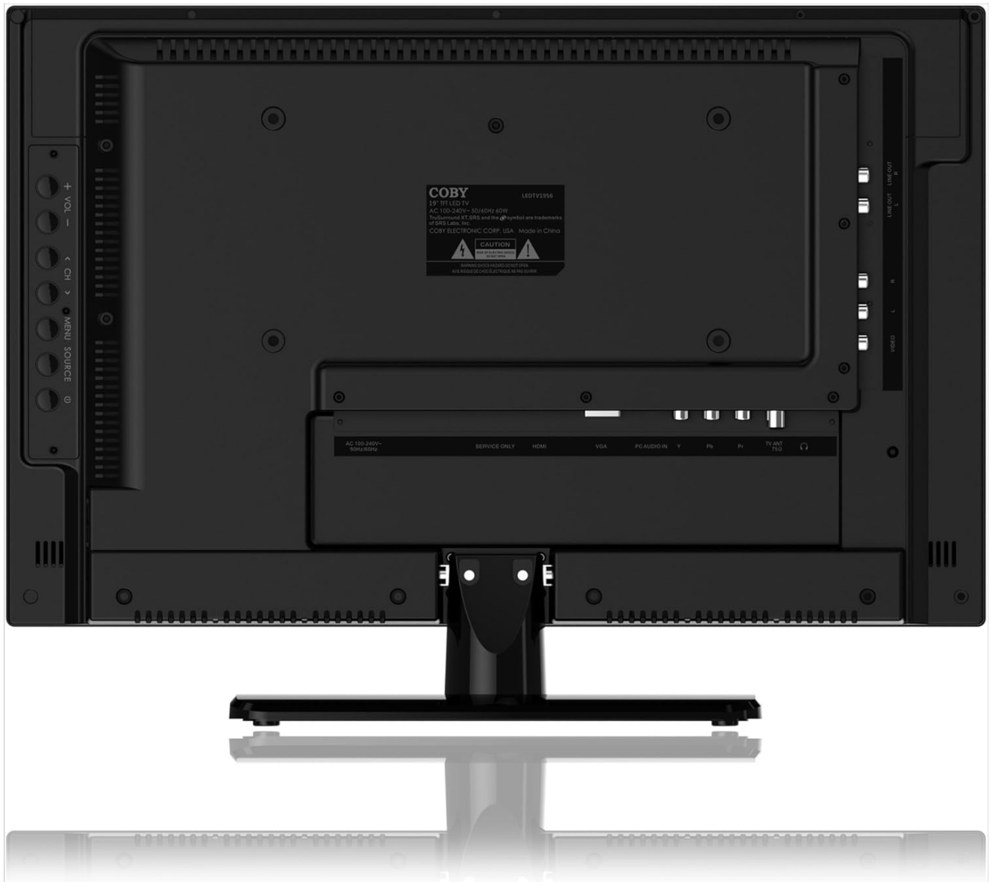
Image: Rear panel of the Coby LEDTV1956 television, displaying input ports including HDMI, VGA, AV, Component, and RF antenna input.
