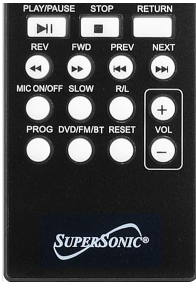
Figure 2: Remote Control for Supersonic SC-37HT. Key buttons include Power, Open/Close, Mute, OSD, Subtitle, Language, Number Pad, Setup, Navigation (Up, Down, Left, Right, Enter), Menu/PBC, Play/Pause, Stop, Return, Rewind, Fast Forward, Previous, Next, Mic On/Off, Slow, Program, DVD/FM/BT (Input Select), Reset, and Volume (+/-).
