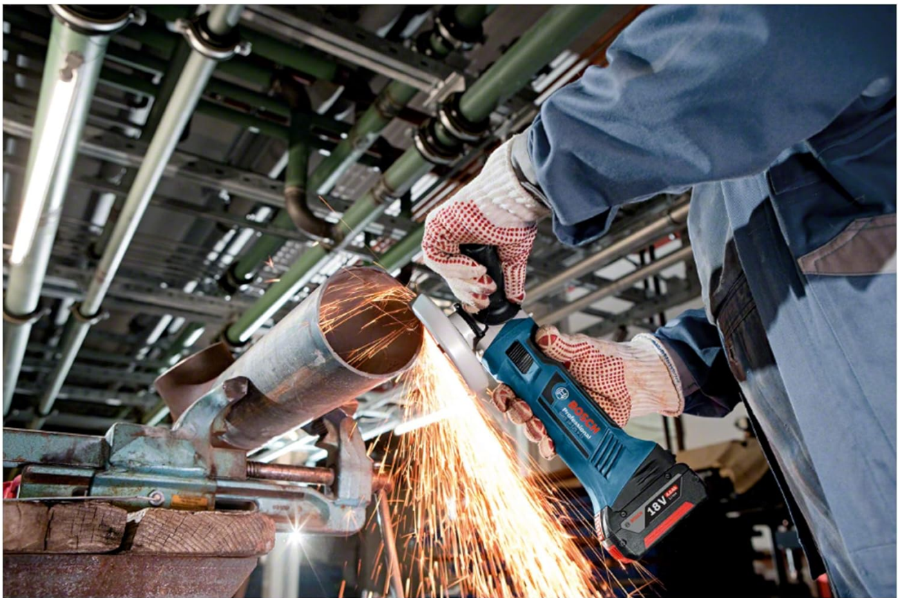
Figure 3: Angle grinder in use cutting a metal pipe. This image demonstrates the tool's capability for precise cutting operations on metal workpieces.
