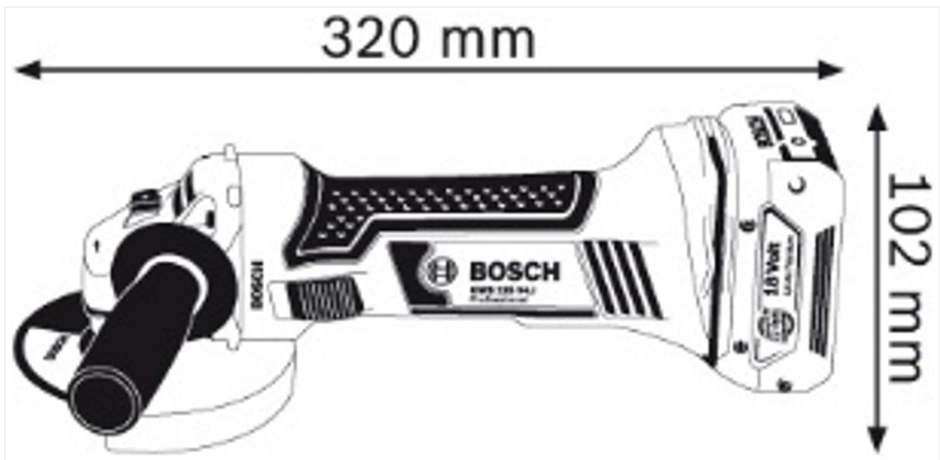
Figure 5: Dimensional drawing of the Bosch Professional GWS 18-125 V-Li. This diagram shows the length (320 mm) and height (102 mm) of the angle grinder.
