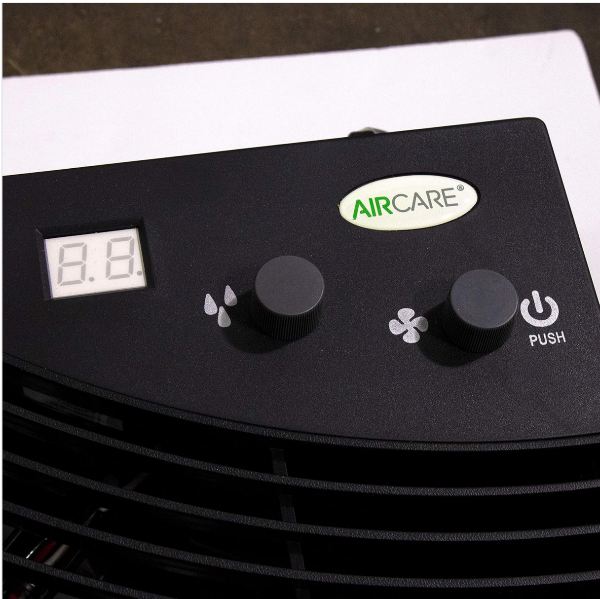
Image 5.1: A close-up view of the digital control panel, showing the humidity control knob, fan speed knob, and power button.
