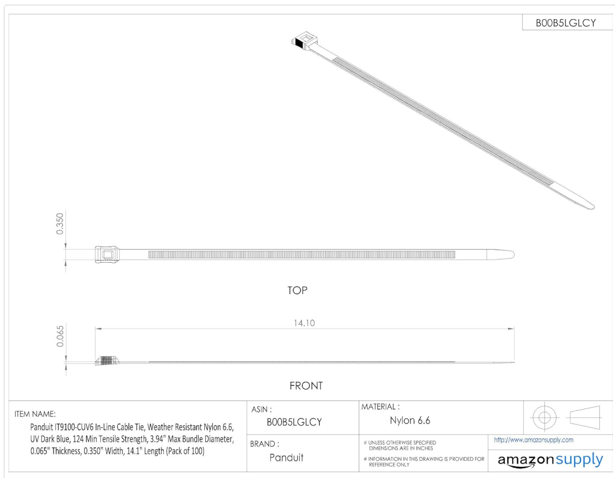
Figure 4: Technical drawing illustrating the dimensions and specifications of the Panduit IT9100-CUV6 cable tie.
